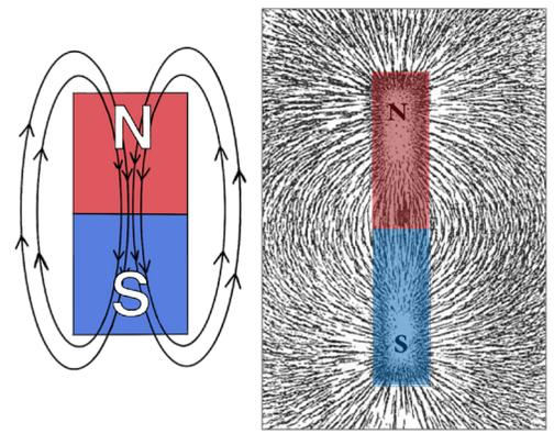
*Left: diagram of the magnetic field of a bar magnet. Right: the magnetic field of a bar magnet revealed by iron filings on paper.*
