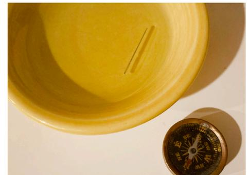
**6.** As a challenge, place the needle with no paper, just using surface tension.
