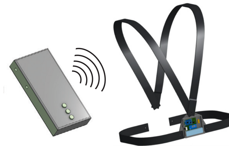
The second Innovation Challenge solution used two custom pieces: a device worn by the referee that emits a radio signal when it perceives a whistle being blown, and a vibrating motor worn on a chest strap by the player.
