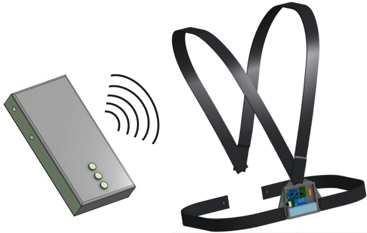
The second Innovation Challenge solution uses two custom pieces: a device worn by the referee that emits a radio signal when it perceives a whistle being blown, and a vibrating motor worn on a chest strap by the player.
