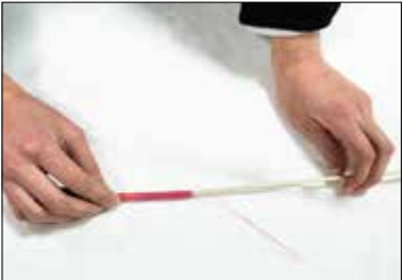
4. Use a skewer to insert a small strip of acetate into the open end of the straw.
